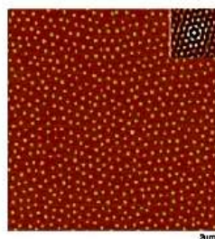
Fig. 1. AFM image of Au particles prepared by a molecular method (10% yield, 20 nm). The inset shows the corresponding autocorrelation function indicating a high degree of hexagonal order. Analysis of the size distribution yields an average diameter of 7.9 \pm 1.2 nm.
