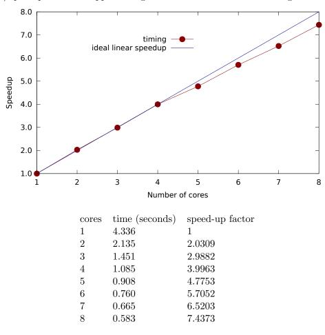
The apparent super-optimal speed-up for two cores is due to inaccurate one-core timing used as a reference.
