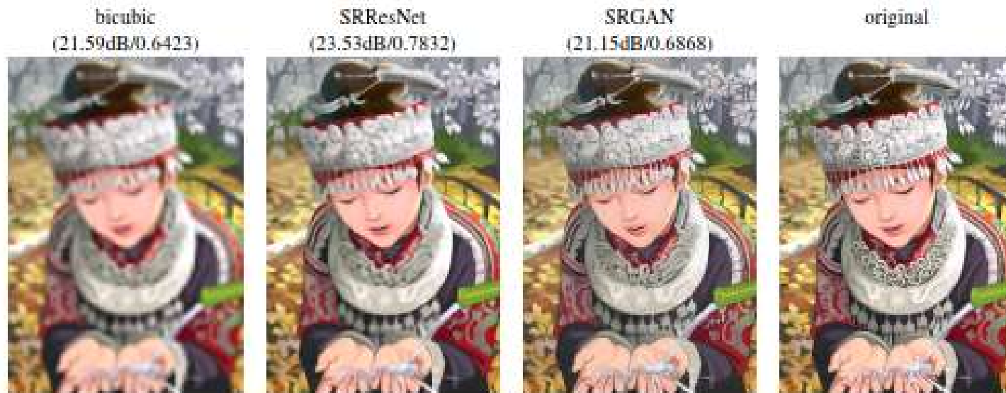
Figure 2: From left to right: bicubic interpolation, deep residual network optimized for MSE, deep residual generative adversarial network optimized for a loss more sensitive to human perception, original HR image. Corresponding PSNR and SSIM are shown in brackets. [4x upscaling]
