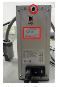
notice that the signal jumps from 0 to 5V, indicating that the Telemed is recording. To stop recording, simply pause the image again and you should see the synchronization signal go from 5V back to 0. Remember to save the ultrasound video. Otherwise, the next time you unpause the device, your video will be lost.
