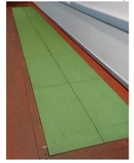
plates). This walkway is effectively 2 rows, each consisting of several force plates laid end to end. It is possible to record force signals from any of the individual plates, but for locomotion purposes, it is more practical to measure the net force from each row separately (or the net force of all plates for running where only 1 limb touches the ground at any given time).
