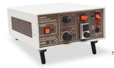
Although you can trigger the Digitimer stimulator manually, I would advise you to trigger it via Spike2, partly because it is more convenient for you, and partly
