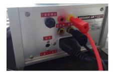
The EMG electrode should be plugged into the preamplifier using the red and yellow ports for active electrodes, and the black port for the reference electrode if available. The amplifier should then be connected to the A/D board by plugging cables into the 'EMG' ports on the back of the amplifier (see figure to the left). The other end of these plugs is a BNC connector that goes to the A/D board.
