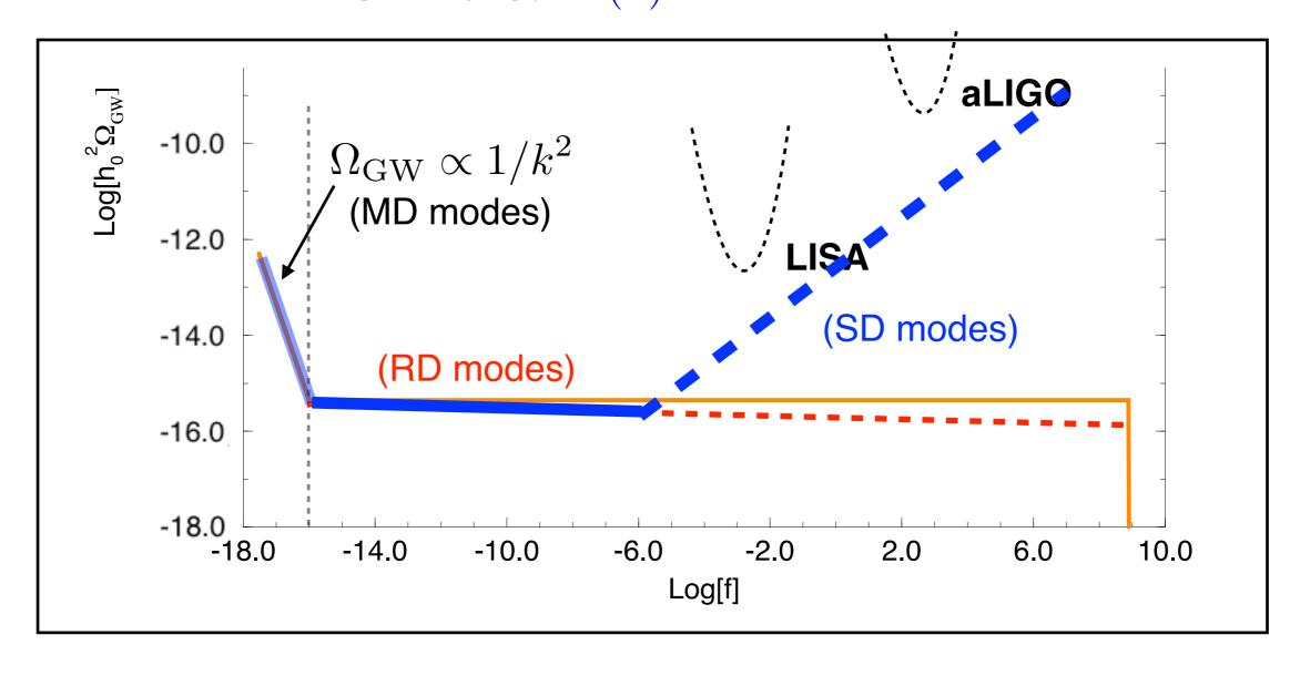
$$\Omega_{\text{GW}}^{(0)}(f) = \Omega_{\text{GW}}^{(0)} \Big|_{\text{plateau}} \times \mathcal{W}(f/f_{\text{RD}}) \times \mathcal{A}_{\text{s}} \left(\frac{f}{f_{\text{RD}}}\right)^{n_t(w_s)},$$
