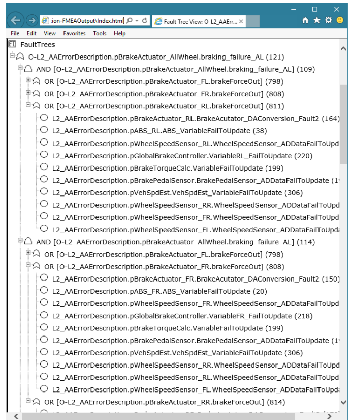
Fig. 7. One of the fault tree and some cut sets generated by HiP-HOPS
