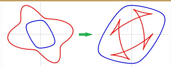
A slowness surface in 2D with its two branches, and the corresponding two Finsler norms. The quasi pressure (qP) polarization behaves well.
