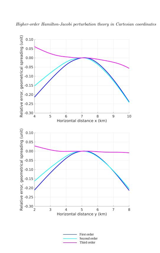
Figure 7. Model VEL: Relative error in geometrical spreading for different extrapolation approaches along the lines y = 5 km (top) and x = 7 km (bottom).
